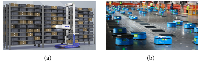
Fig. 1. MAPD applications: (a) an automated fulfillment center with robots carrying multiple objects [6]; (b) an automated sortation centre [7].
